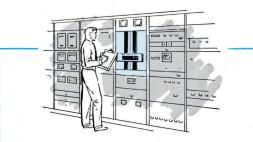
The design of the PB 250 enables it to be mounted as a systems component in  $31\frac{1}{2}$  in. of a standard relay rack.
