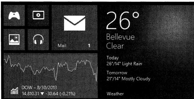
FIGURE 8-2 The Start screen showing four small tiles (top left), one medium tile (with "Mail" as the branding name and "1" as the badge), one wide tile (bottom left, with a branding logo), and one large tile (with "Weather" as the branding name).
