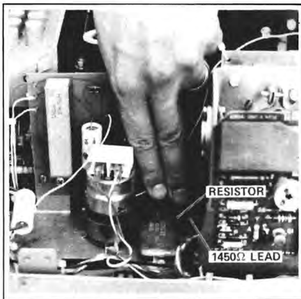
Figure B-2. Current Source Resistor
