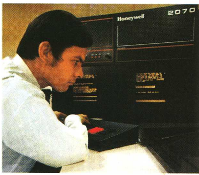
Operator control with OS/2000 and the Type 220-8 CRT Console.
