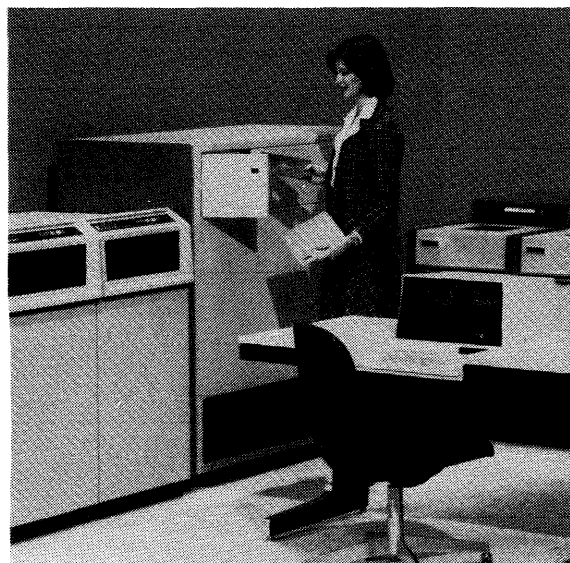
The Criterion Series firmware is loaded via flexible disks, as shown here. Different sets of firmware enable the system to duplicate the operating characteristics of the earlier NCR century systems, or to operate as a COBOL 74 virtual machine. Also shown is the standard console display unit and keyboard.
