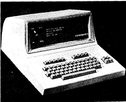
serial lines or 75 KB/second parallel lines. There are six special functions: bell, line feed, return, delete, tabbing, and a configuration flow chart. The 401 is priced at \$1495 in single quantity, and delivery is 60 days ARO. The 401 can be used with the manufacturer's model 101 line printer. For information:
