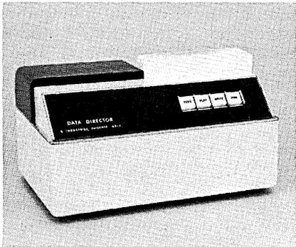
A 3½ x 7⅝-inch card can store more than 26,000 bits. Visual information can be written or typed on the non-magnetic portion of the cards. Interfacing to any minicomputer or terminal is accomplished through a standard interface. The Data Director sells for \$1880. B INDUSTRIES, INC., Phoenix, Ariz. For information:
