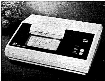
with units containing Russian, Hebrew, Greek, or other character sets. And the printer is said to be quiet enough to place in an office environment, printing an entire 8 x 10-inch page in 20 seconds. The line length is 80 columns. The RS-232-compatible printer can handle asynchronous data rates up to 50 Kilobaud. The price for the DI-240 is \$4100, and deliveries are scheduled for July. DATA INTERFACE ASSOCIATES, Danbury, Conn. For information:
