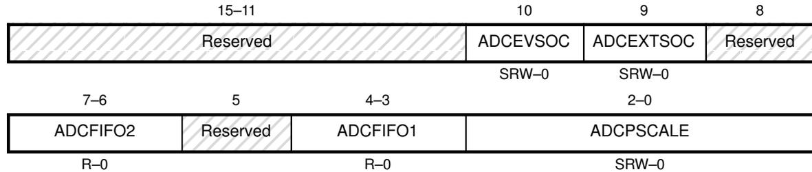
**Note:** R = read access, W = write, S = shadowed, –0 = value after reset
